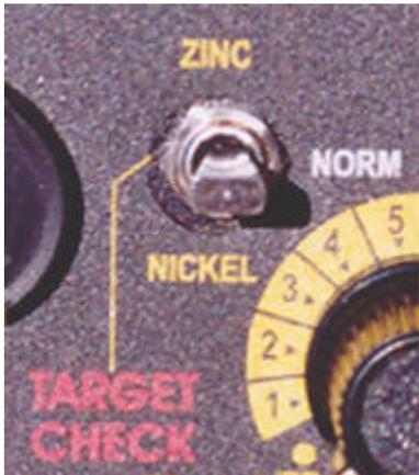
Here is a feature of the Shadow X5 that coinshooters will absolutely love. The TARGET CHECK is a three-position switch. When the switch is pushed up (ZINC) or down (NICKEL) it will always return to the center position (NORM) because it is spring loaded.
