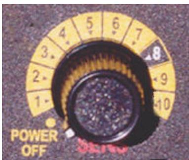
level of sensitivity of the detector. The Sensitivity adjustment will have a huge affect on the performance of the X5. The general thinking of some coinshooters is to crank up the sensitivity to the max and start hunting. Well, that may not work with the X5. The X5 SENS control is designed so that a setting of “9” will be so sensitive that you will start experiencing a chirping sound. Remember, you are dealing
