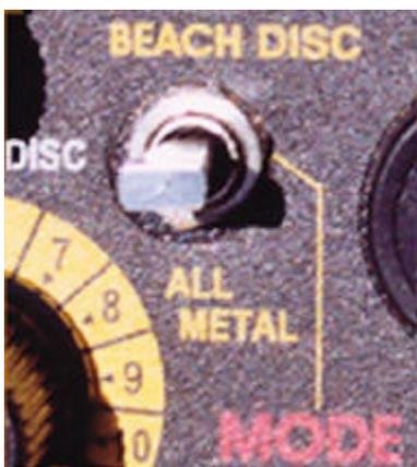
1. There is the fast auto-tune all-metal motion search mode. This is the normal All Metal mode with which most of us are familiar. It will require a small amount of coil motion to detect a target.
